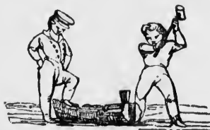
Fig. 307.—APPLICATION OF THE WEDGE.
